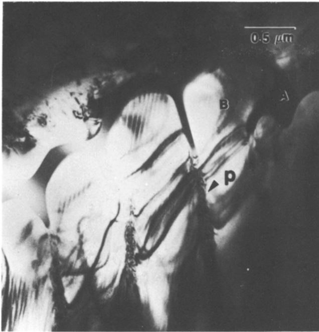
Figure 7 TEM micrograph of BaO-doped \alpha' - C_2S showing grain boundary phase (A), grain (B) and precipitates (p).
