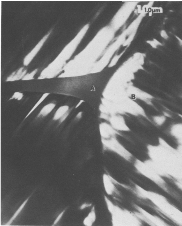
Figure 5 TEM micrograph of P_2O_5 -doped \beta - C_2S showing grain boundary phase (A) and grain (B).
