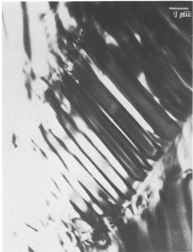
Figure 6 TEM micrograph of B_2O_3 -doped \beta - C_2S showing a domain structure.
